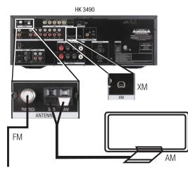
Figure 13 – Antenna Connections
